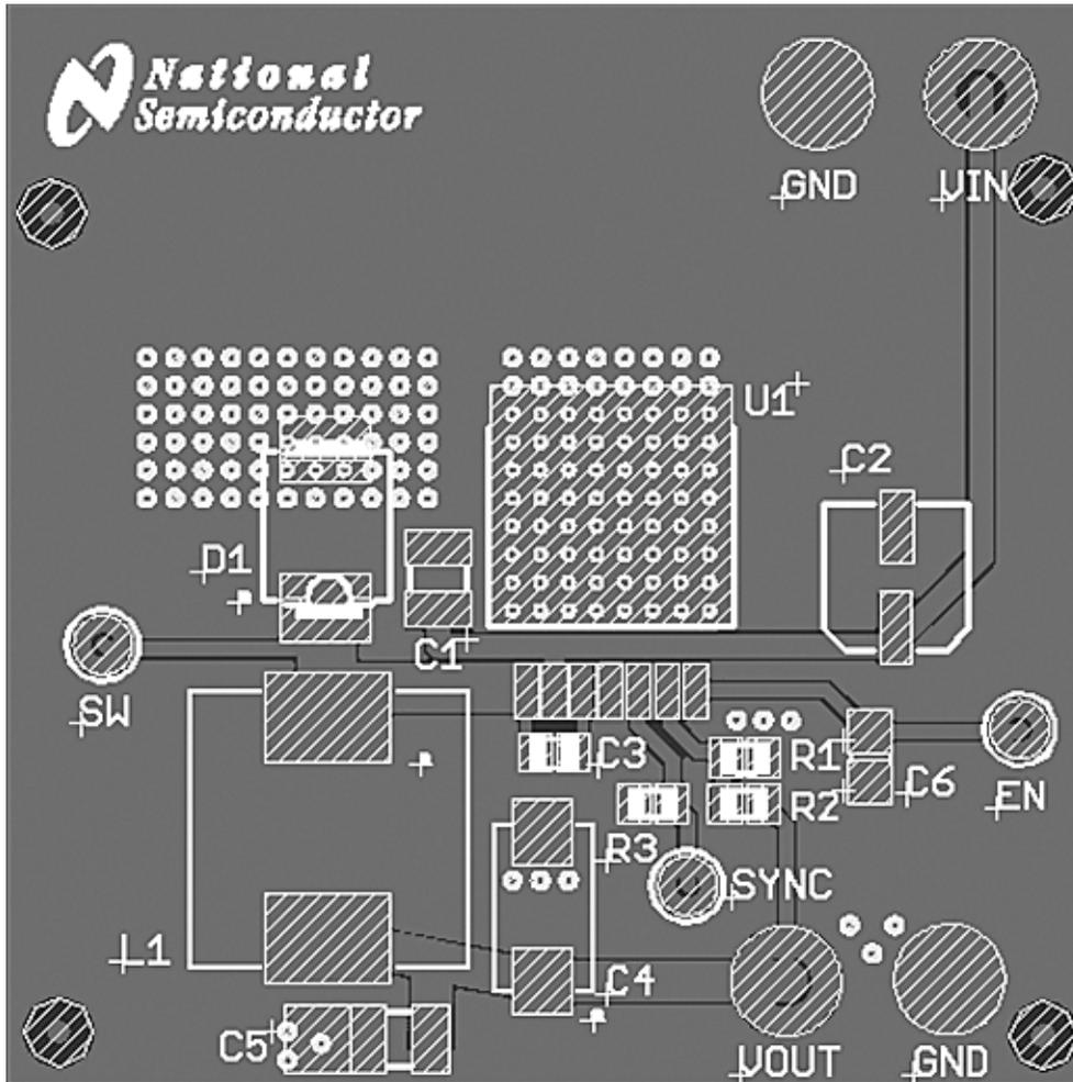
PCB Layout Example for PSOP-8 Package
