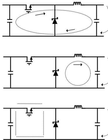
**Figure 13. Current Flow in a Buck Application**
