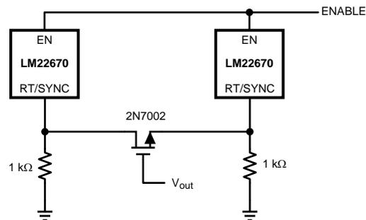
Figure 9. Self Synchronization Set up
