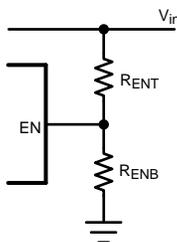
**Figure 4. External UVLO Connections**
