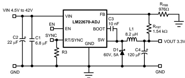
Figure 11. Typical Buck Regulator Application
