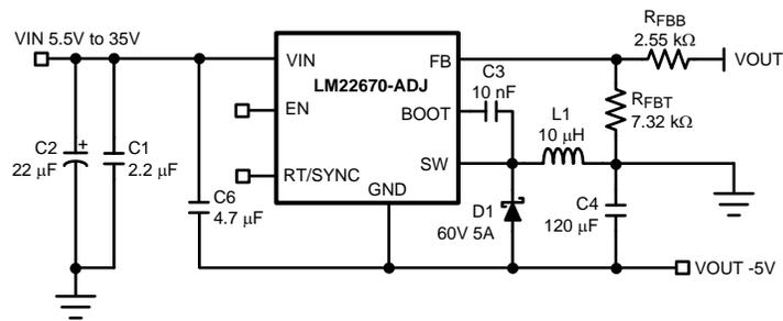
Figure 14. Inverting Regulator Application
