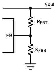
**Figure 12. Resistive Feedback Divider**
