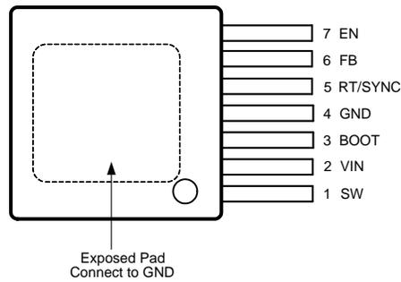
**Figure 2. 7-Lead Plastic TO-263 THIN Package**
