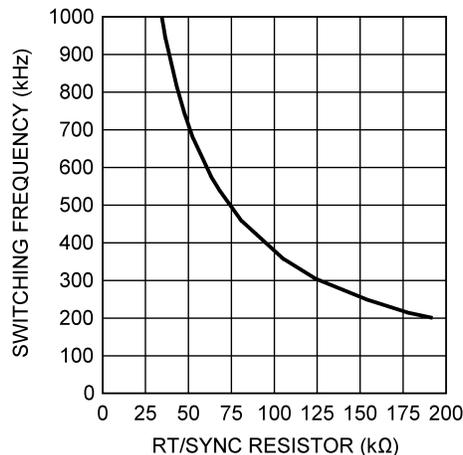
**Figure 8. Switching Frequency vs RT/SYNC Resistor**
