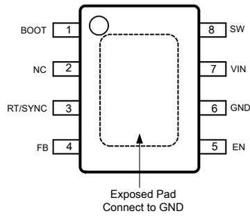
**Figure 1. 8-Lead Plastic PSOP-8 Package**
