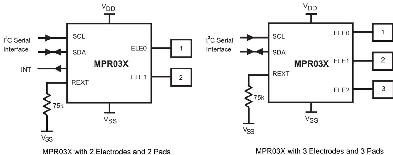
Figure 13. MPR03X Pad and Interrupt Connection Options
