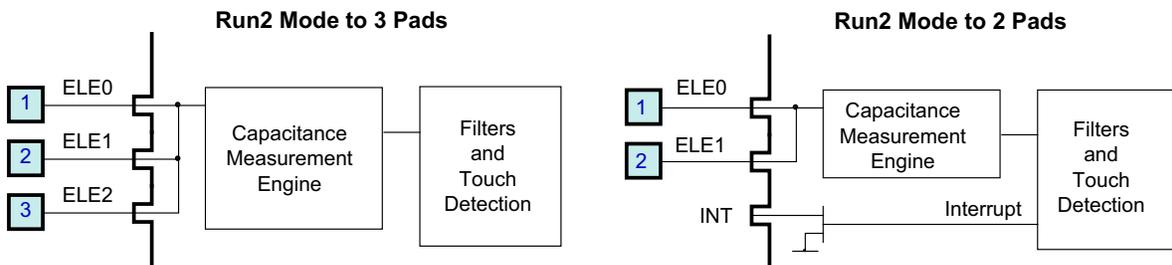
Figure 15. Electrode/Pad Connections in Area Detection Mode
