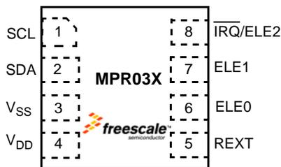
**Figure 3. Package Pinouts**
