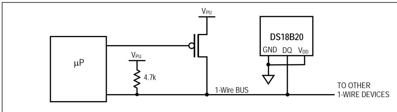
**Figure 5. Powering the DS18B20 with an External Supply**
