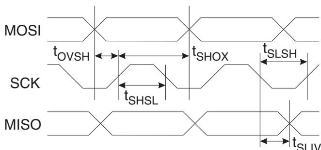
**Figure 29-4.** Serial Programming Waveforms
