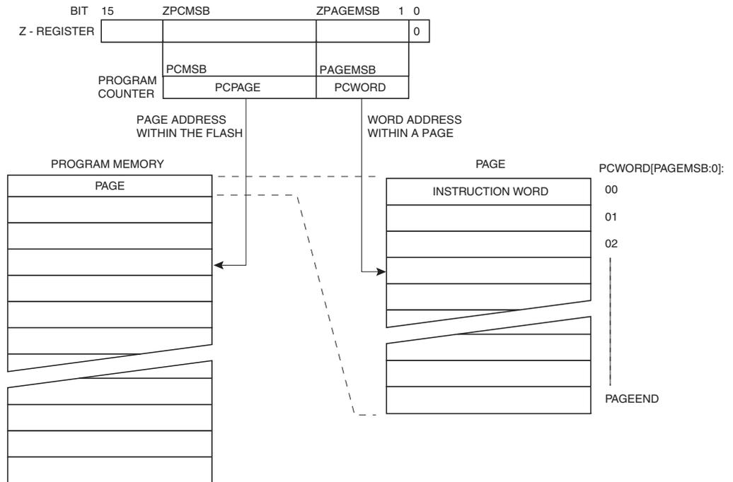
Note: 1. The different variables used in [Figure 27-1](#) are listed in [Table 28-7 on page 183](#).
