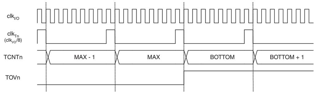
Figure 20-10 on page 99 shows the setting of OCF0B in all modes and OCF0A in all modes except CTC mode and PWM mode, where OCR0A is TOP.
