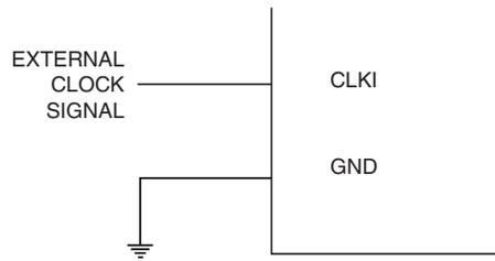
When this clock source is selected, start-up times are determined by the SUT Fuses as shown in [Table 14-8 on page 46](#).
