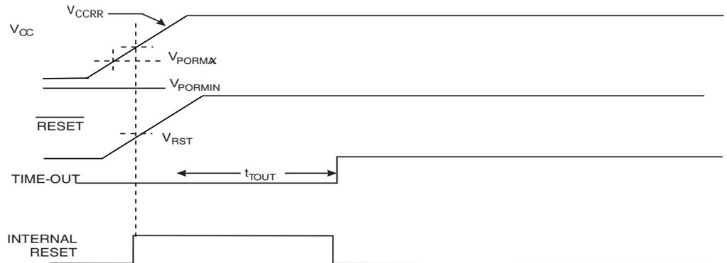
**Figure 16-3.** MCU Start-up,  $\overline{\text{RESET}}$  Extended Externally
