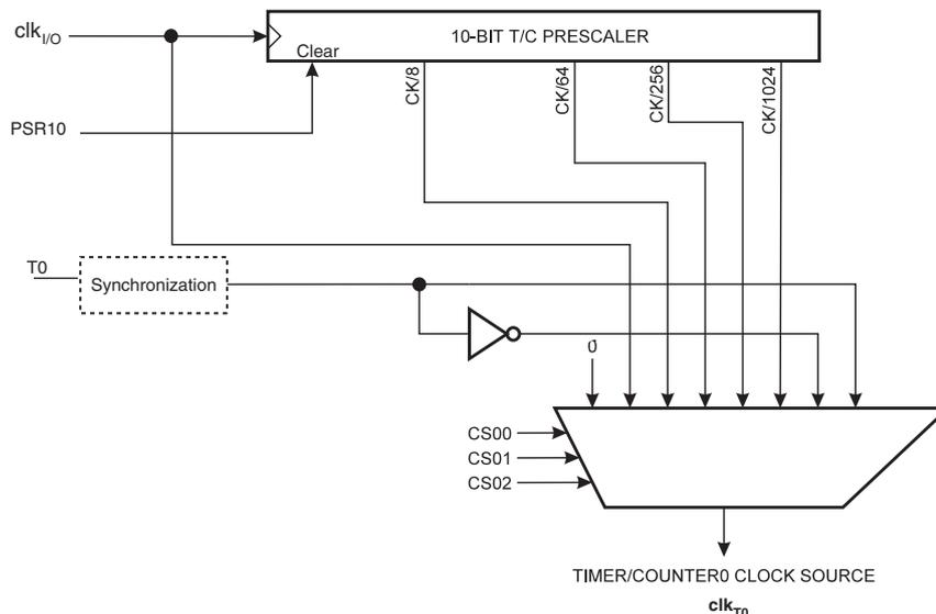
Note: 1. The synchronization logic on the input pins (T0) is shown in [Figure 22-1 on page 136](#).
