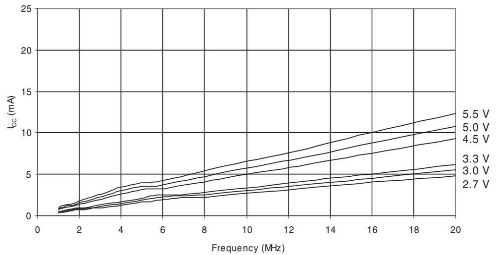
Figure 30-4. Active Supply Current vs. frequency (1 - 20 MHz) - Temp.=125°C
