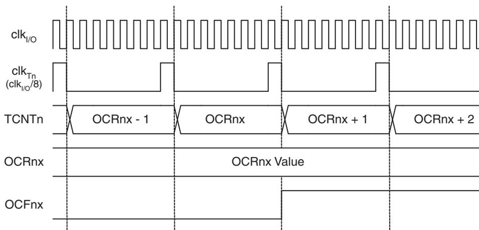
Figure 21-12 on page 127 shows the count sequence close to TOP in various modes. When using phase and frequency correct PWM mode the OCR1x Register is updated at BOTTOM. The timing diagrams will be the same, but TOP should be replaced by BOTTOM, TOP-1 by BOTTOM+1 and so on. The same renaming applies for modes that set the TOV1 flag at BOTTOM.
