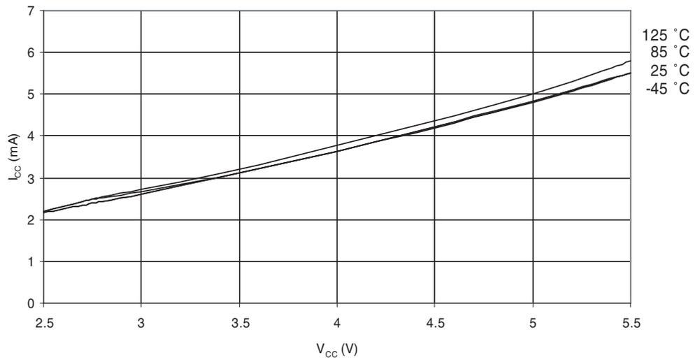
**Figure 30-6.** Active Supply Current vs.  $V_{CC}$  (Internal RC Oscillator, 1 MHz)
