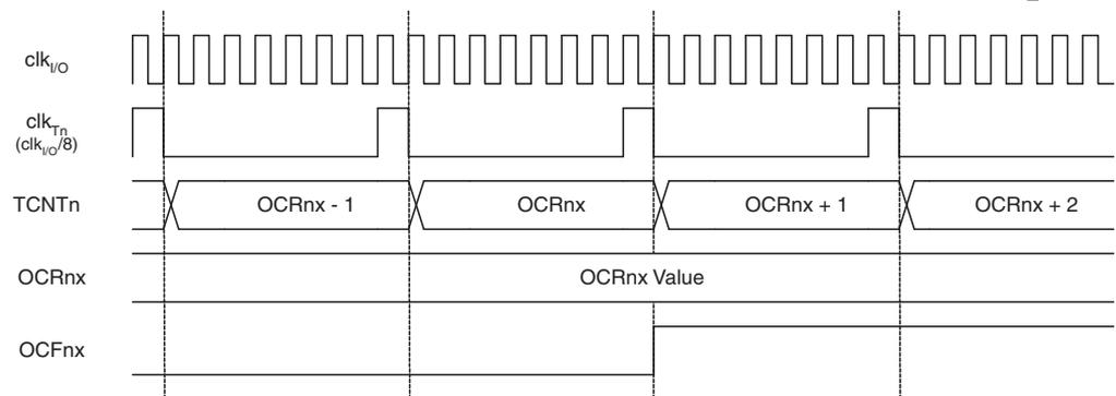
Figure 20-11 on page 99 shows the setting of OCF0A and the clearing of TCNT0 in CTC mode and fast PWM mode where OCR0A is TOP.
