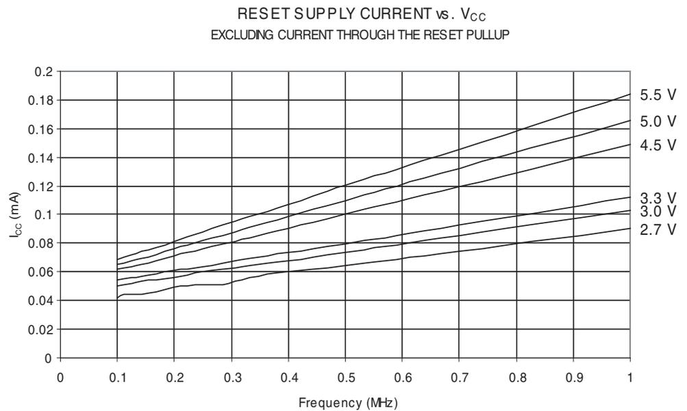
**Figure 30-43.** Reset Supply Current vs.  $V_{CC}$  (1 - 20 MHz, Excluding Current Through the Reset Pull-up)
