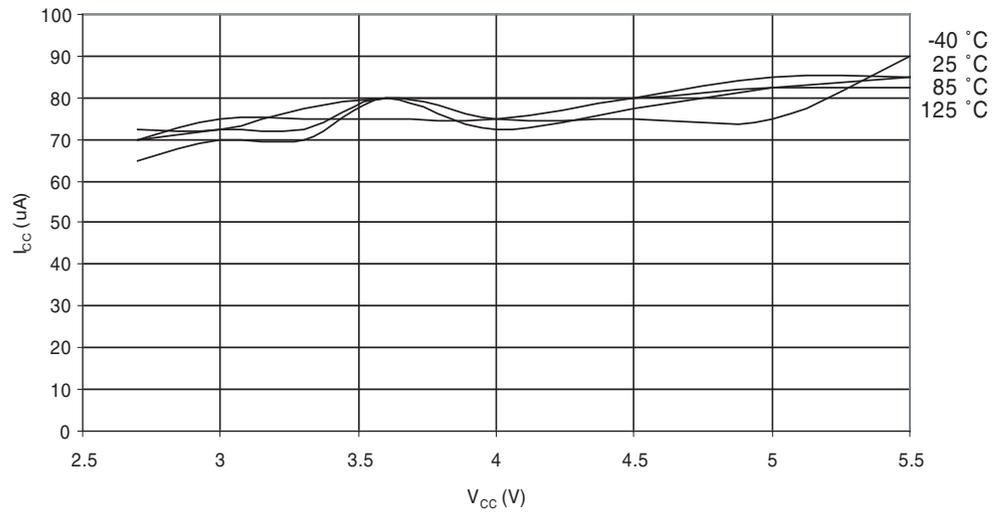
Figure 30-39. Programming Current vs.  $V_{CC}$
