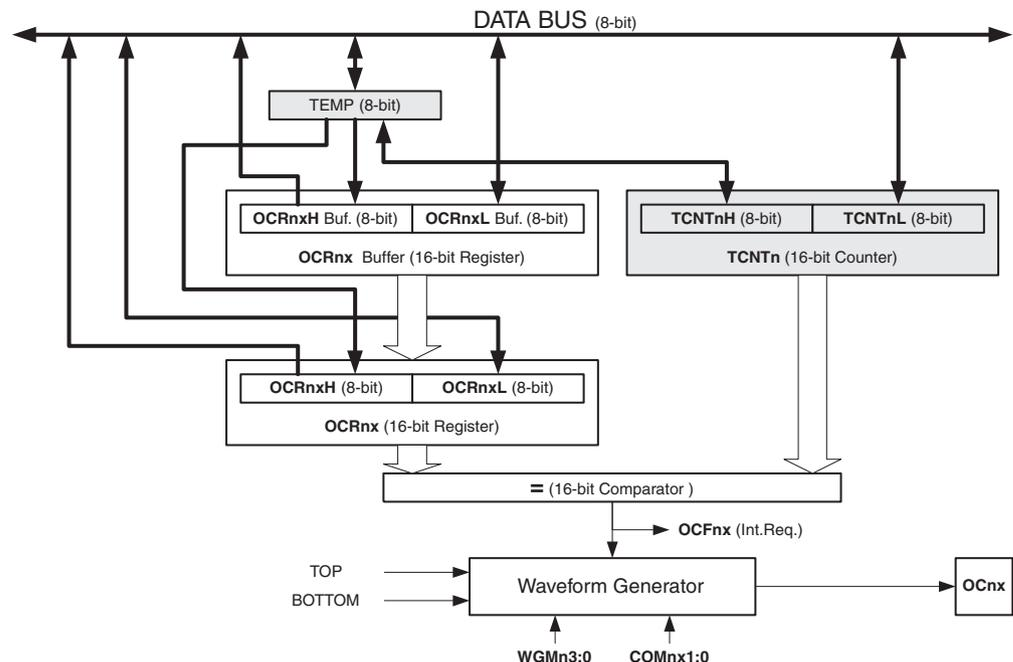
The OCR1x Register is double buffered when using any of the twelve *Pulse Width Modulation* (PWM) modes. For the Normal and *Clear Timer on Compare* (CTC) modes of operation, the double buffering is disabled. The double buffering synchronizes the update of the OCR1x Compare Register to either TOP or BOTTOM of the counting sequence. The synchronization
