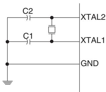
The Oscillator can operate in three different modes, each optimized for a specific frequency range. The operating mode is selected by the fuses CKSEL3..1 as shown in [Table 14-3 on page 43](#).
