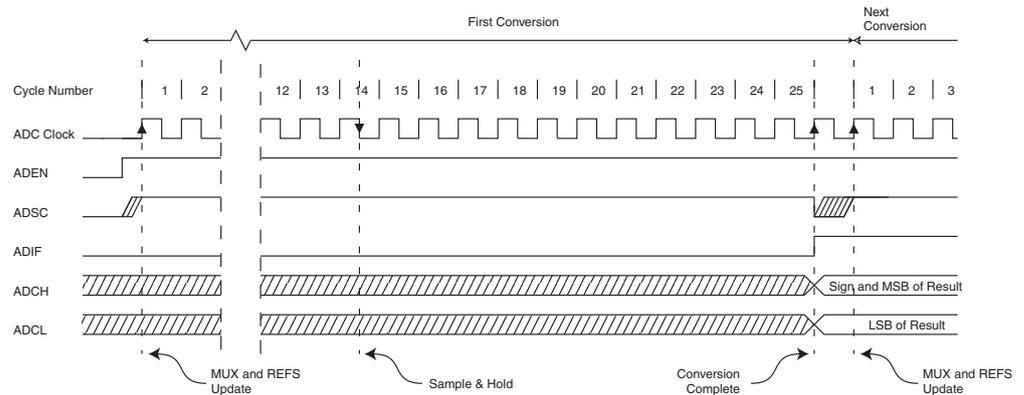
**Figure 25-5.** ADC Timing Diagram, Single Conversion
