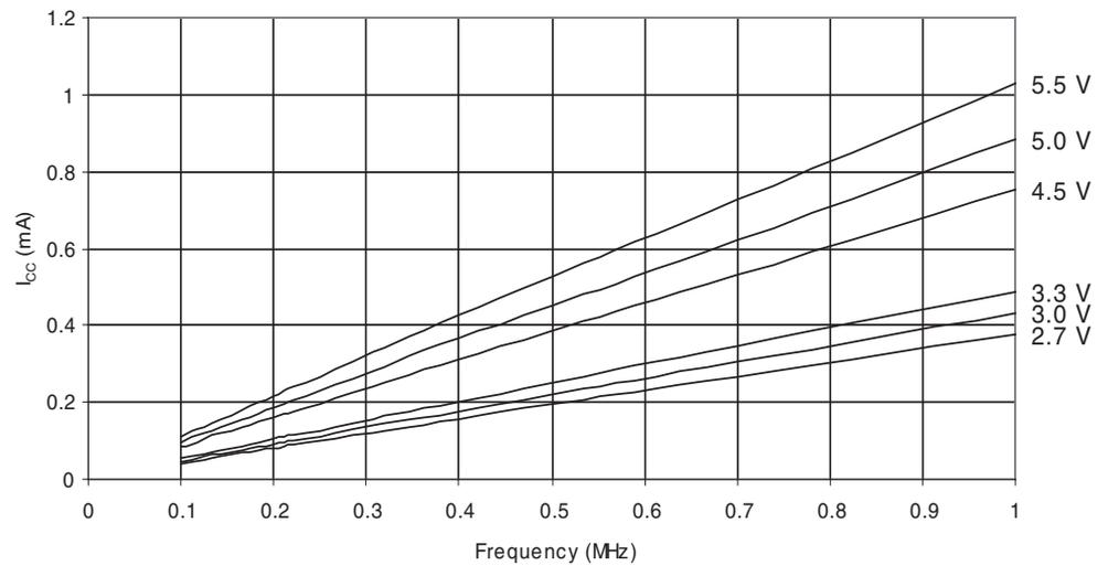
Figure 30-3. Active Supply Current vs. frequency (1 - 20 MHz) - Temp.=25°C
