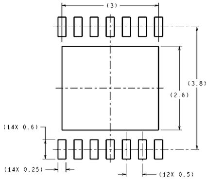
**DIMENSIONS ARE IN MILLIMETERS**
