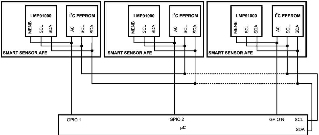
**FIGURE 9. SMART GAS SENSOR AFES on I<sup>2</sup>C bus**
