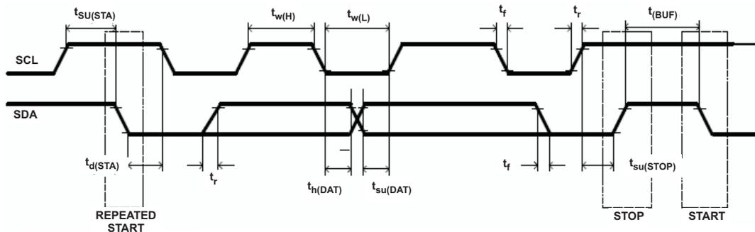
Figure 4. I<sup>2</sup>C-Compatible Interface Timing Diagrams
