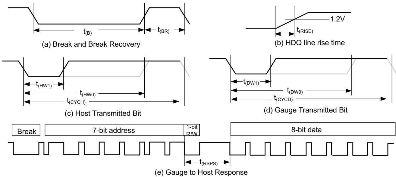
Figure 3. Timing Diagrams
