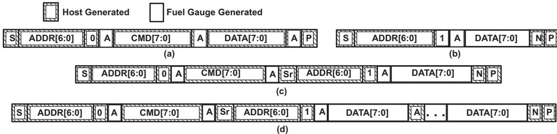
**Figure 6. Supported I<sup>2</sup>C formats: (a) 1-byte write, (b) quick read, (c) 1 byte-read, and (d) incremental read (S = Start, Sr = Repeated Start, A = Acknowledge, N = No Acknowledge, and P = Stop).**
