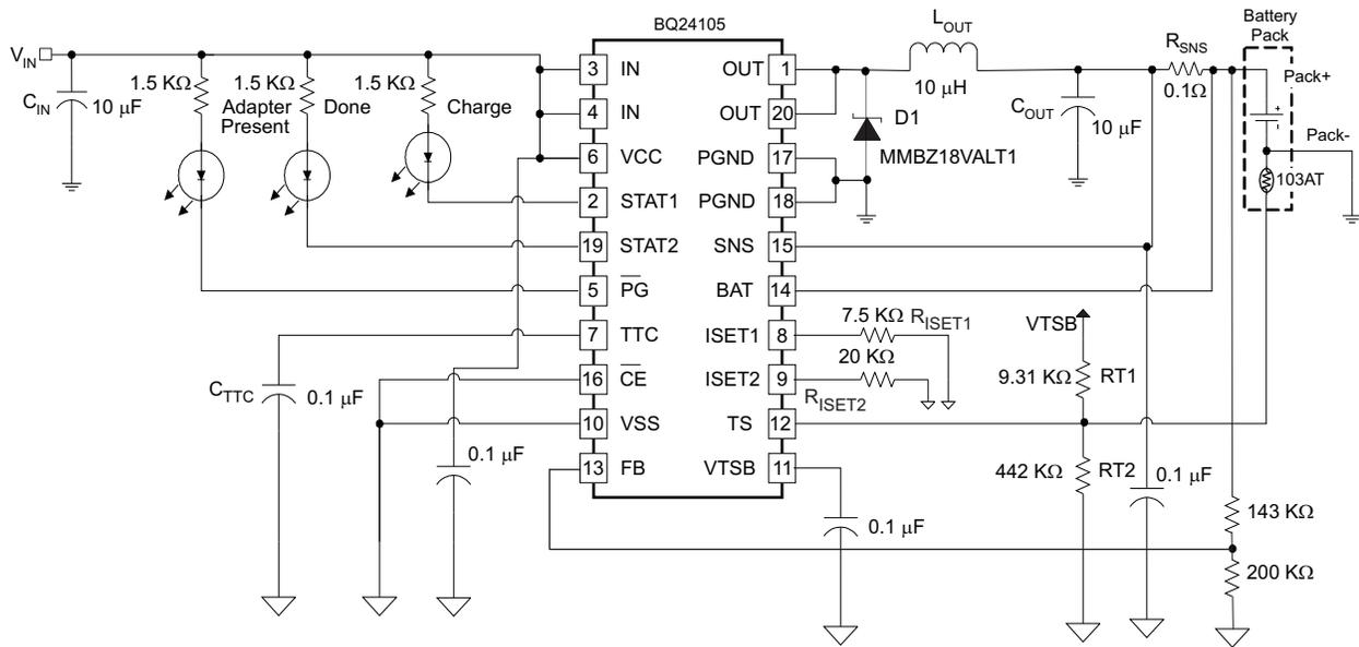
Figure 19. 1-Cell LiFePO<sub>4</sub> Application
