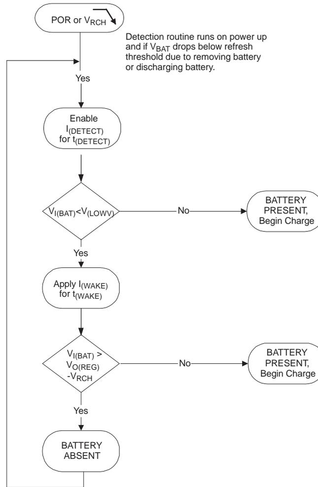
Figure 11. Battery Absent Detection for bq2410x ICs only
