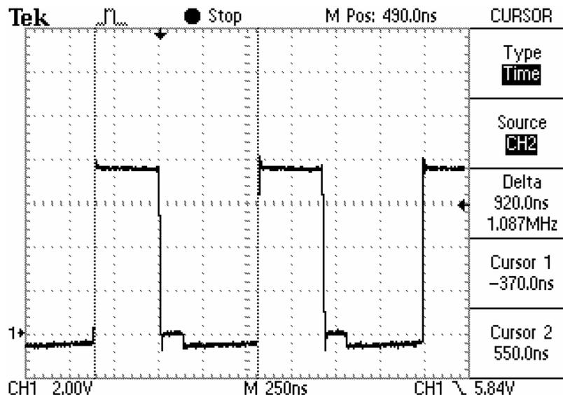
Precharge: The current is low in precharge; so, the bottom synchronous FET turns off after its minimum on-time which explains the step between X0 V and -0.5 V. When the bottom FET and top FET are off, the current conducts through the body diode of the bottom FET which results in a diode drop below the ground potential. The initial negative spike is the delay turning on the bottom FET, which is to prevent shoot-through current as the top FET is turning off.
