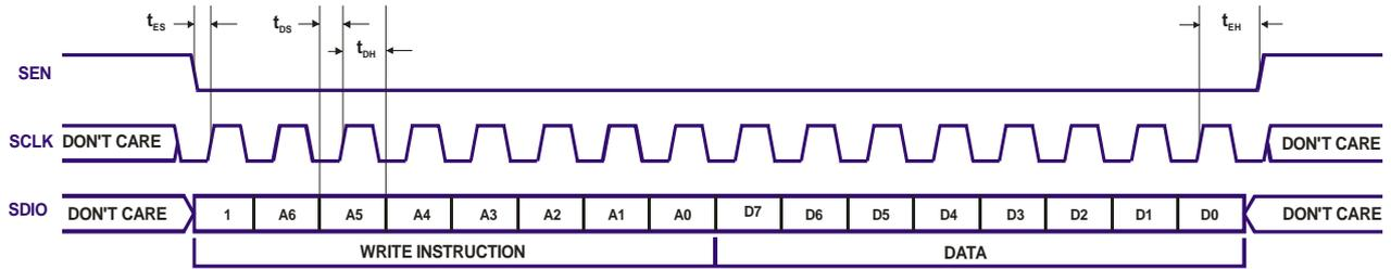
Figure 14: SPI write cycle, 3-wire and 4-wire modes
