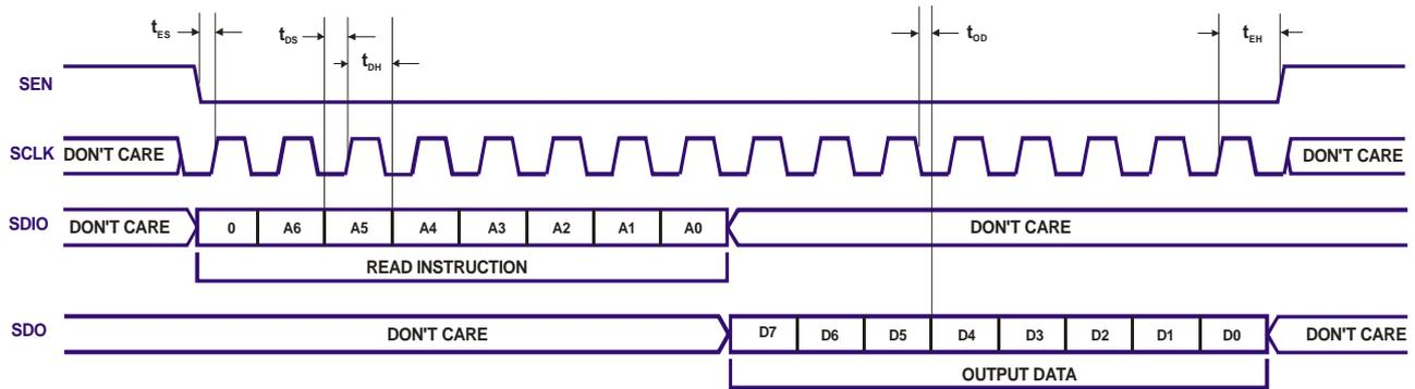
Figure 15: SPI read cycle, 4-wire mode (default)
