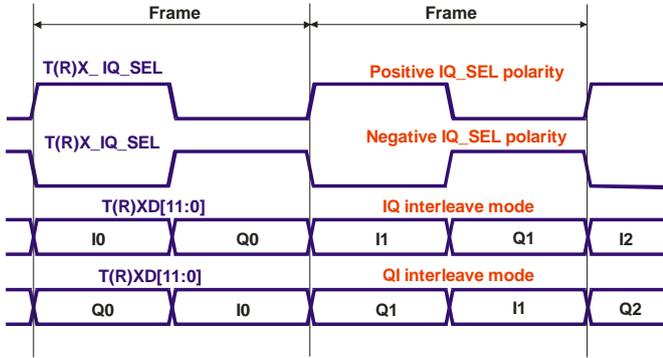
Figure 8: Frame sync polarity and interleave modes
