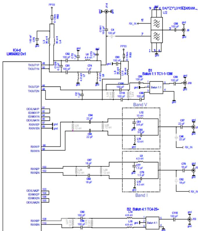
Figure 19: LMS6002D Typical Application Circuit Diagram – RF part
