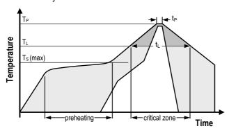
**Figure 5:** Soldering profile according to JEDEC standard.  $T_P \le 260^{\circ}\text{C}$  and  $t_P \le 40\text{sec}$  for Pb-free assembly.  $T_L \le 220^{\circ}\text{C}$  and  $t_L \le 150\text{sec}$ . Ramp-up/down speeds shall be  $\le 5^{\circ}\text{C/sec}$ .
