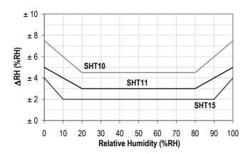
Figure 2: Maximal RH-tolerance at 25°C per sensor type.
