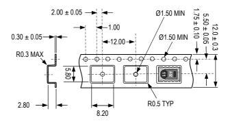
**Figure 21:** Tape configuration and unit orientation within tape, dimensions in mm (1mm = 0.039inch). The leader tape is at the right side of the figure while the trailer tape is to the left (direction of unreeling).
