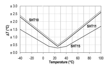
Figure 3: Maximal T-tolerance per sensor type.
