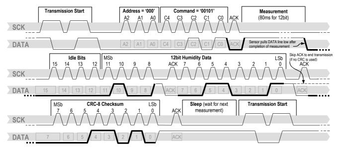
**Figure 17:** Example RH measurement sequence for value "0000'0100"0011'0001" = 1073 = 35.50%RH (without temperature compensation). DATA valid times are given and referenced in boxes on DATA line. Bold DATA lines are controlled by sensor while plain lines are controlled by the micro-controller.
