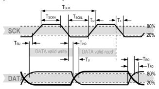
**Figure 11:** Timing Diagram, abbreviations are explained in Table 3. Bold DATA line is controlled by the sensor, plain DATA line is controlled by the micro-controller. Note that DATA valid read time is triggered by falling edge of anterior toggle.
