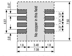
Figure 7: Recommended footprint for SHT1x. Values in mm.
